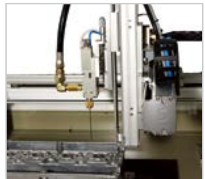
▲ 3 Axis Robot Bonding For Car Engine Cover
