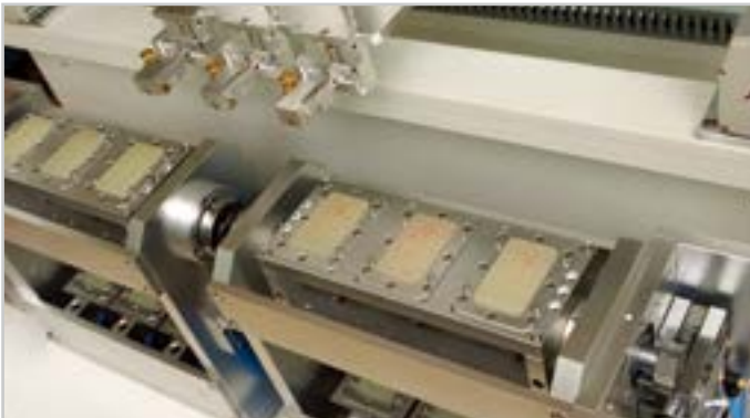
▲ 3 Axis Robot Keypad Bonding By Press Unit
