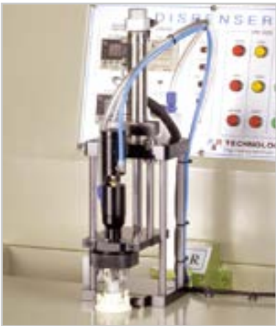
▲ 2K Epoxy Mult Potting By UpDown Unit
